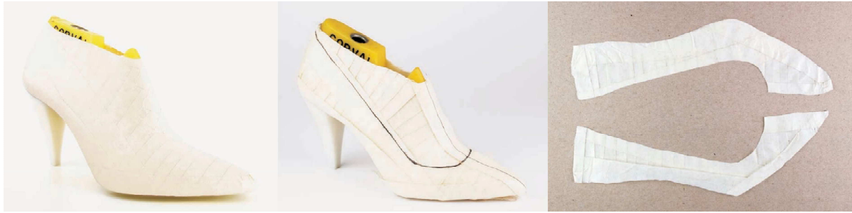
Figure 1. Process of shoe-last-based footwear product development [2].
