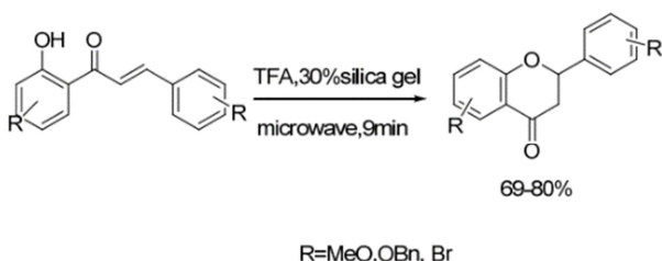
Figure 28. Microwave Accelerated Solvent-Free Synthesis of Flavanone.
